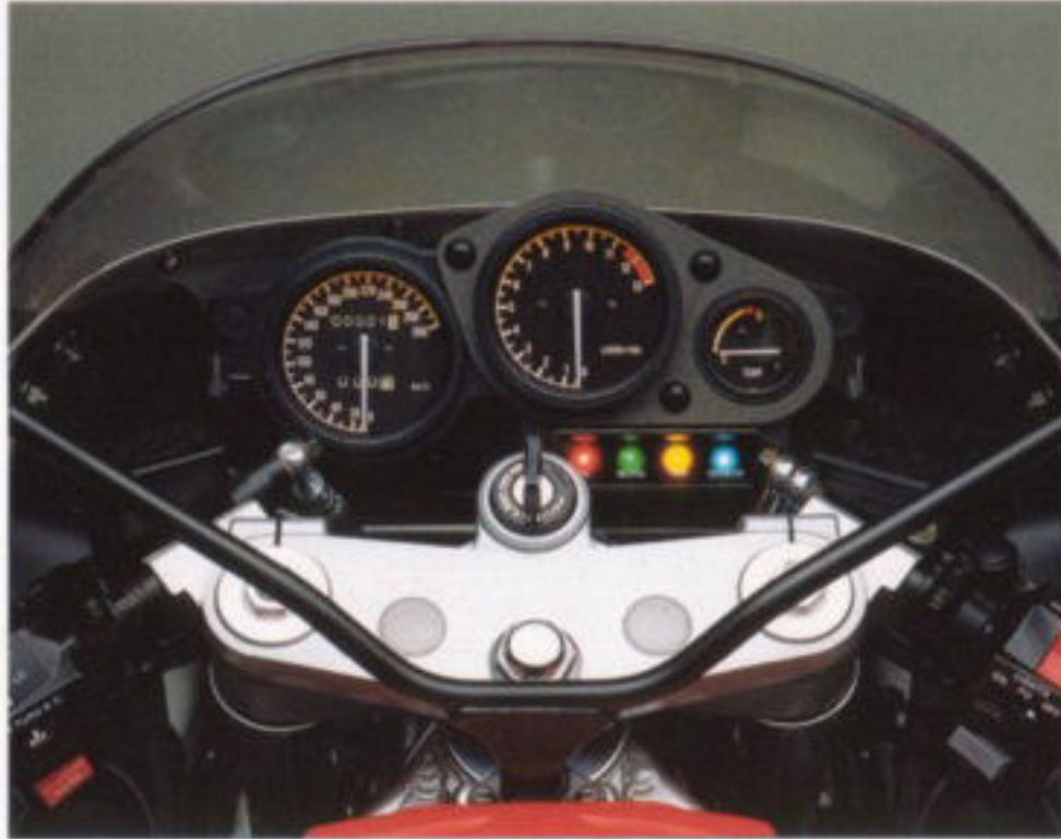
Instrument panel Fairing-mounted instrument panel houses the tachometer, speedometer and water temperature gauge. Easy-read dials and warning lights provide instant information at a glance, allowing the rider to concentrate fully on the road ahead.
