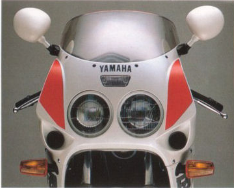
Fairing/FAI Super aerodynamic fairing incorporates flush-fitting headlights for reduced drag. Twin FAI (Fresh Air Intake) scoops funnel cool, dense air directly into the airbox and carburettors for optimum engine performance throughout the whole speed range.
