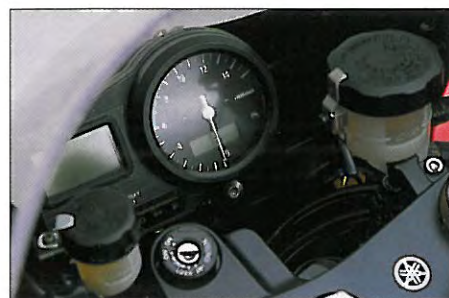
Clocks are strictly business with analogue rev counter and liquid crystal displays for everything else
