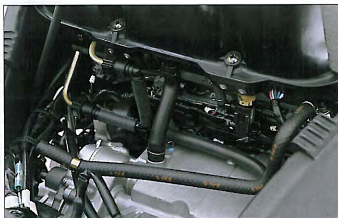
The R7 differs from the R1 and R6 in its fuelling – the R7 is equipped with fuel injection (rather than carbs) which sits just below the airbox
