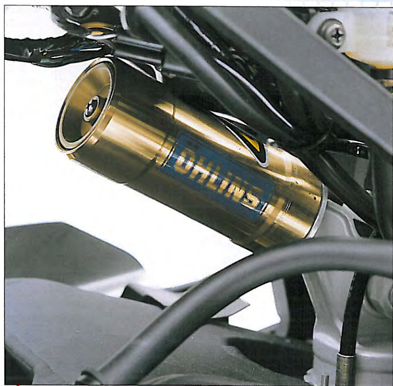
The Öhlins rear suspension unit is operated by a linkage system from the swingarm
