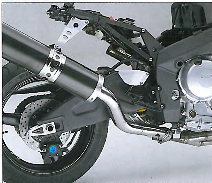
The engine on the Yamaha is exceptionally stiff too, with the result that the chassis overall is one of the strongest available on any road bike
