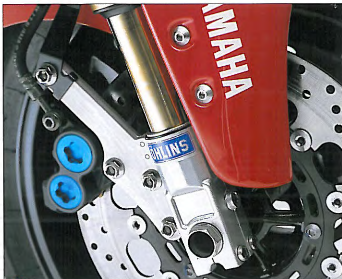
The forks are Öhlins inverted racing items with a very low friction titanium alloy coating, which is the gold finish you see here
