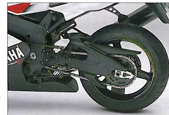
The rear suspension, along with an extended swingarm, features a fully adjustable piggyback type Ohlins shock absorber
